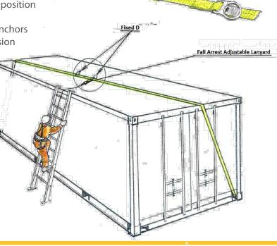
SAFE WORKING LOAD (SWL) Rated for two(2) person use, end anchors shall be rated to 21kN
